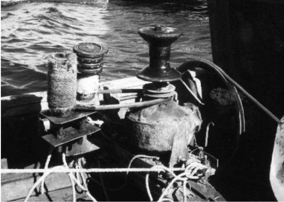
Typical boat winch with rope coiler
