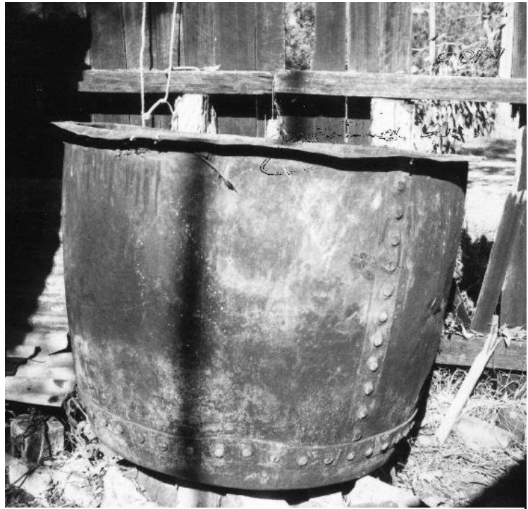
A tanning pot used to coat cotton nets with tannins from boiled ironbark so that they would not rot
