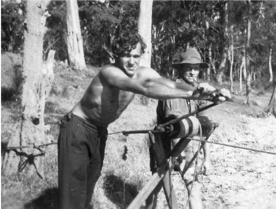
Allan (Casey) Wynn and Gus Williams c1948 using a two handed winch to haul net. Note winch lashed to tree. Serious injuries from the steel handles were common if they were released, allowing them to spin backwards at great speed.
