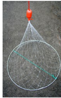
A 'witches hat' – the float keeps the netting material off the bottom and the inverted mesh operates as an entanglement net.
